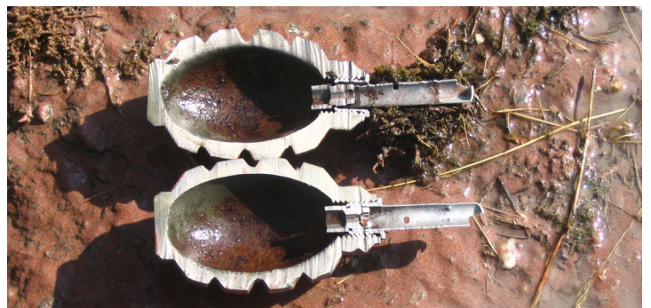
A cut of a hand grenade
