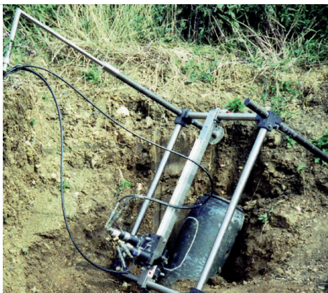
Cutting a burn out hole with 3-axis cutting table
