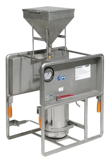
The AMU 700-12 is an Abrasive Mixing Unit and part of a water jet cutting system for safe and efficient cutting using the water abrasive suspension (WAS) technique. It is particularly suitable for mobile applications.
