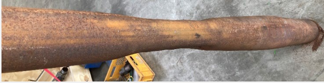
4.5" Tubing test fixture with collapse
