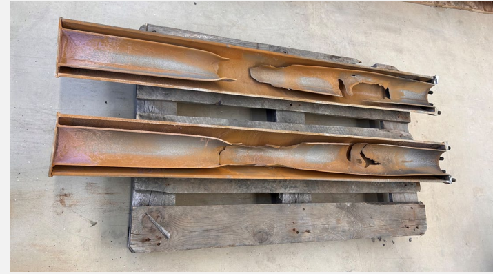
4.5" Tubing test fixture cut in half
