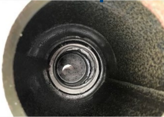
Stuck flow target coil tubing
