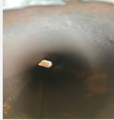
4.5" Tubing test fixture with collapse
