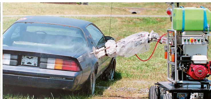
miniMACE in use with EOD robot
