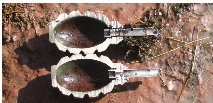
A cut of a hand grenade
