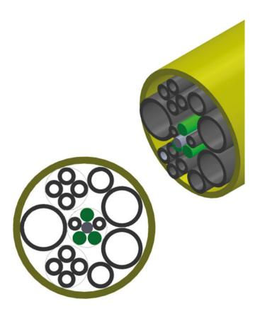
The ANT Work Umbilical is a durable and reliable supply line for WAS-cutting with ANT's offshore cutting equipment (DCH, PCH). It is built as a fully housed umbilical with a protective, 5 mm thick TPE layer.
