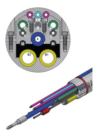
The ANT Test Umbilical is designed for workshop - testing and function tests. The umbilical is ready for packer operations. The velcro jacket allows for replacement of single hoses and cables.
