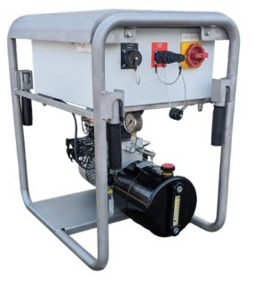
The MACE hydraulic system enables effective control of cutting devices of the Water Abrasive Suspension (WAS) cutting unit MACE. An intuitive operator panel enables precise control of motion axes and cutting speed. It allows for safe, remote controlled operation from up to 500 m distance, even at difficult operating conditions.
